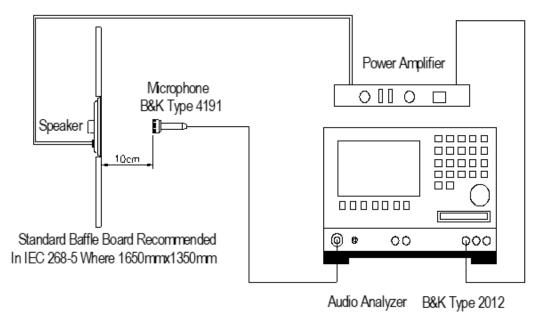
Typical Frequency Response (Temperature: 23 ~ 25 °C; Humidity: 55% max; Power: 0.1W, 10cm)
