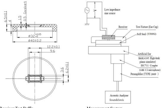
Receiver Test Baffle
