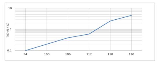
Microphone Output versus SPL Input (with acoustic source at 50cm)
