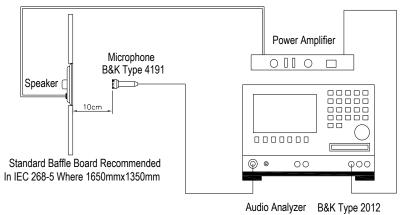
Frequency Response (measured with 2.45V @ 10cm in 1cc enclosure)
