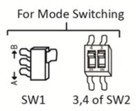
The input method can be set to single-ended (V0-p) inputs or differential (Vp-p) inputs and is controlled by dip switches 1 and 2 on SW2.
