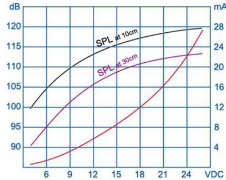
SPL & Current Consumption vs. Input Voltage
