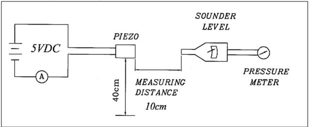
**Reliability Testing** Standard Test Condition (+5~+35°C, 45~85% RH) Judgement Test Condition (+25±2°C, 60~70% RH)
