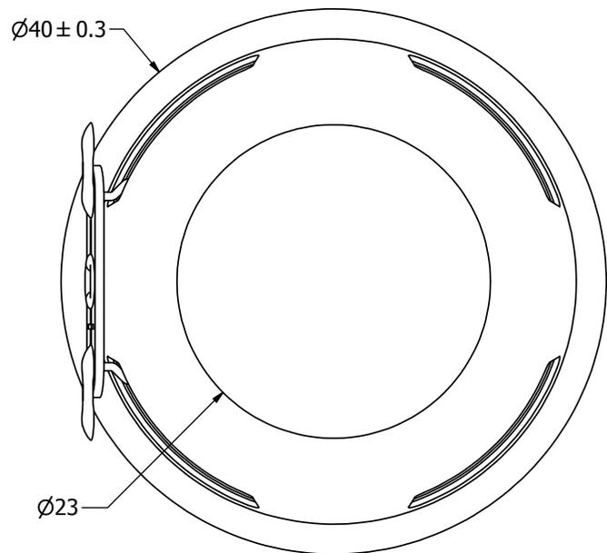
ALLOW AT LEAST 0.8mm FOR DIAPHRAGM MOVEMENT (ø35.6 BAFFLE OPENING)
