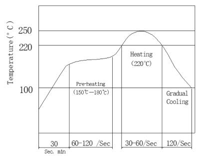
\*Manual Soldering – Iron temp 350C, Solder Time 3 second or less.
