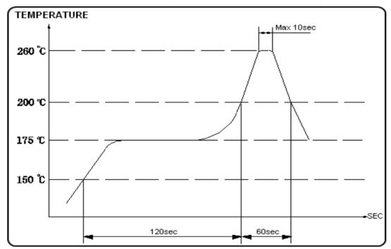
\* Hand Soldering temperature 350°C within 5 sec.
