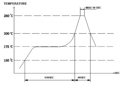
\*Manual soldering with 350C iron temp and 2-3 seconds solder time per terminal.
